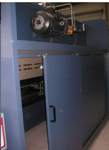
Rear safety doors
