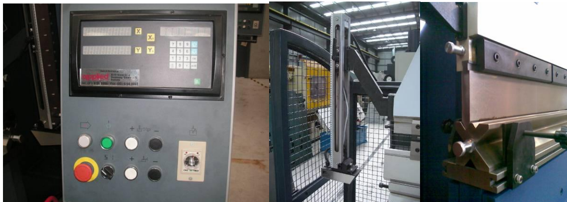
Basic DRO controller for (NC) pressbrake Laser safe guarding 200T standard tooling
