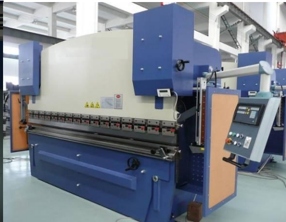
CPB pressbrake with hydraulic crowning
